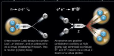
A free neutron (udd) decays to a proton (uud), an electron, and an antineutrino via a virtual (mediating) W boson. This is neutron  $\beta$  (beta) decay.
