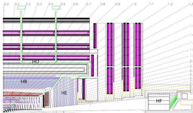
Figure 3.10: Longitudinal view of the CMS detector showing the locations of the hadron barrel (HB), endcap (HE), outer (HO) and forward (HF) calorimeters.
