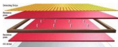
Figure 3.14: Resistive Plate Chambers
